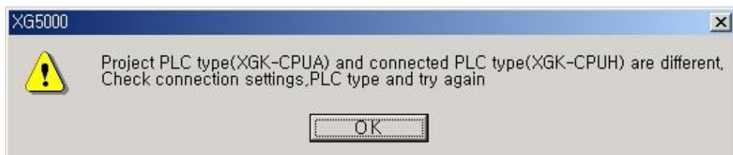
[Fig. 6.2.6] [CPU type is incorrect]
